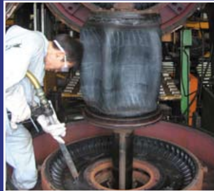
Clean hard to reach areas in tire molds.
