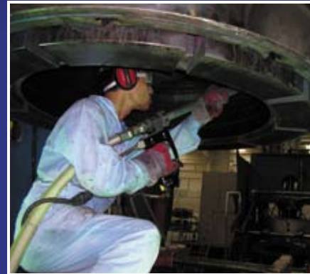
Clean hard to reach areas in tire molds.
