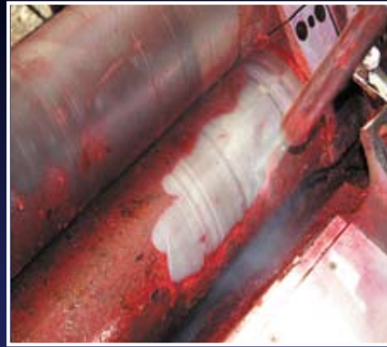
The Cold Jet solution is non-abrasive and won't harm equipment.
