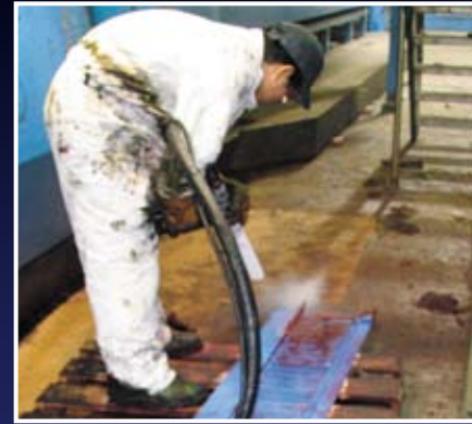
The Cold Jet solution is non-abrasive and won't harm equipment.
