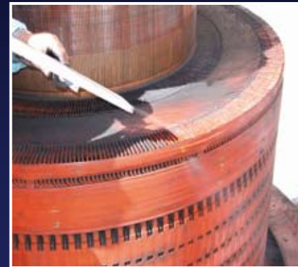
Clean conductive equipment with a non-conductive process.
