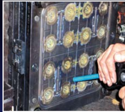
Clean molds hot and in place with Cold Jet Dry Ice Blasting.
