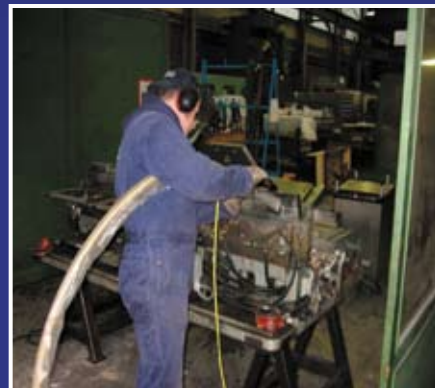
Cold Jet's non-abrasive process will not damage molds.
