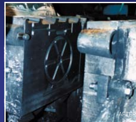
Before and after cleaning with a Cold Jet dry ice blasting system.
