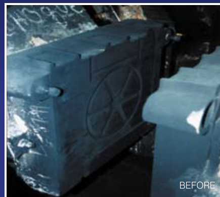
Before and after cleaning with a Cold Jet dry ice blasting system.
