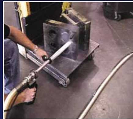
Remove harmful release agent from permanent molds.
