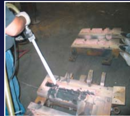
Remove harmful release agent from permanent molds.
